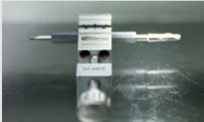
After manufacturing product (fixture), Dimension of product is tested by non-contact visual microscope to measure precise dimension.
