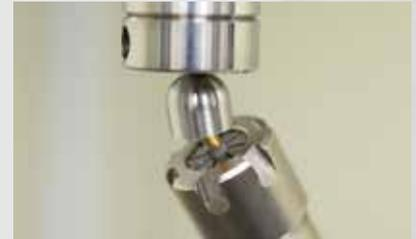
For providing the strength of product and a long-term safety, a fatigue test is done by measuring a mechanical force. Based on ISO14801:2016, the test is taken place.
